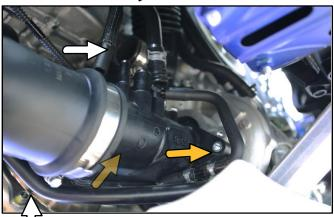
4) Remove the diverter vacuum hose from the car and replace with the hose supplied with the GFB Respons TMS kit.
