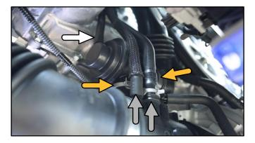
3) Using a 10mm socket, remove the two bolts that hold the turbo intake pipe onto the turbo.
