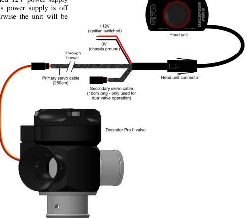
Often there is an existing grommet that can be used for this purpose. In any case, it is important to ensure that the lead is protected where it passes through the firewall to prevent wear or damage.
